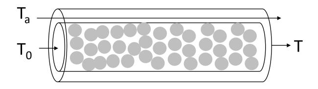
For a packed bed reactor, we may use catalyst weight (W) instead of reactor volume (V)
