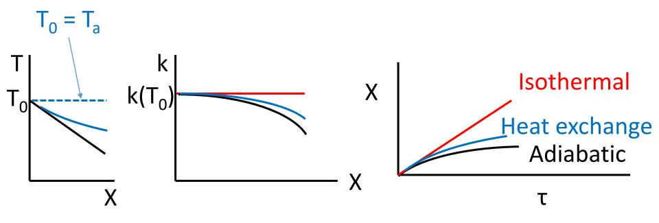
For a heat exchanger with coolant, what if coolant temperature  $(T_a)$  is not constant?
