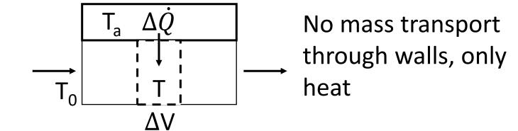
Reactor with coolant/heating adjacent to reactant volume.  $\dot{Q} \neq 0$ . In reactant slug have a  $\Delta \dot{Q}$  term from V to V+ $\Delta$ V.
